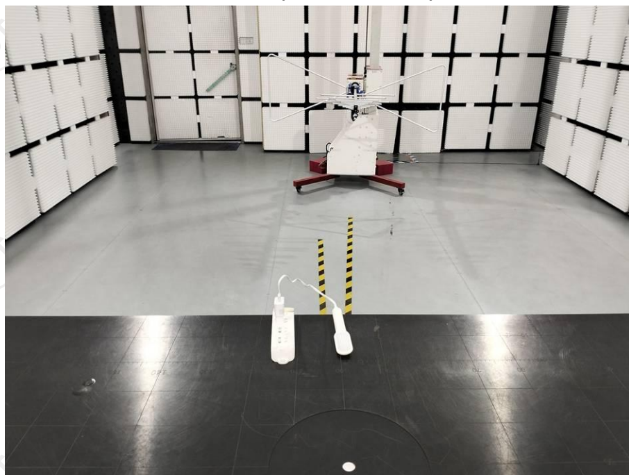
Radiated emission (30 MHz to 1 GHz) Test View
