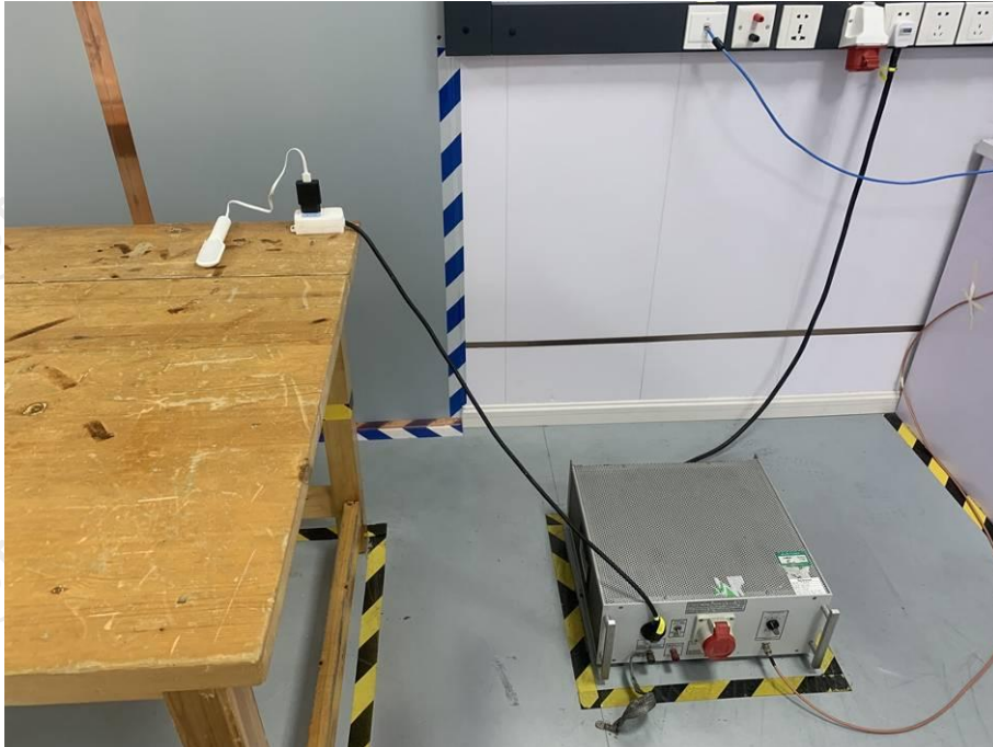
Disturbance voltage at mains terminals test view
